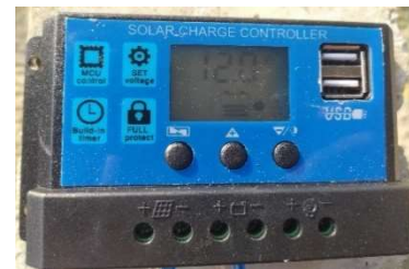
Gambar 5. Solar Charger Controller
